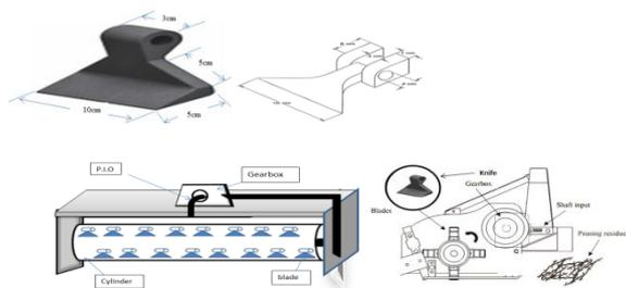
**Figure 1.** Machine for shredding orchard tree waste
