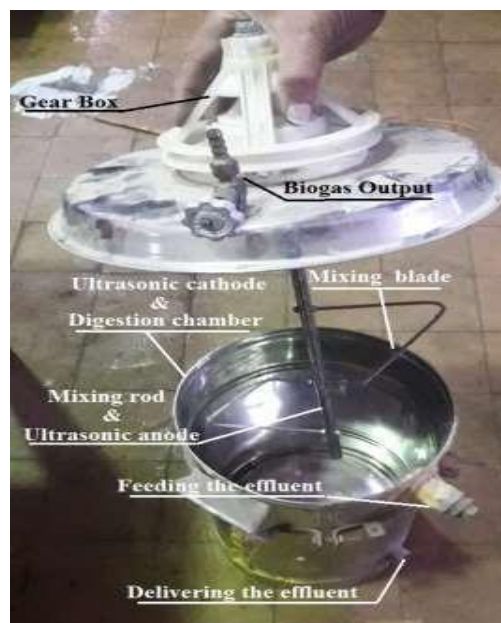
Fig. 2 The digestion chamber and biogas outlet pipes.
