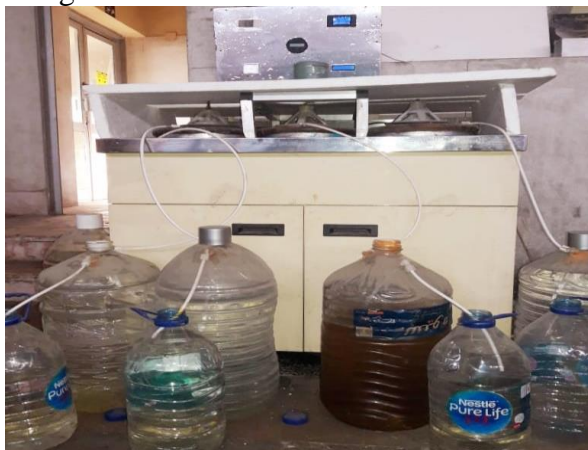
Fig. (1a) Microwave Anaerobic Digester System.
